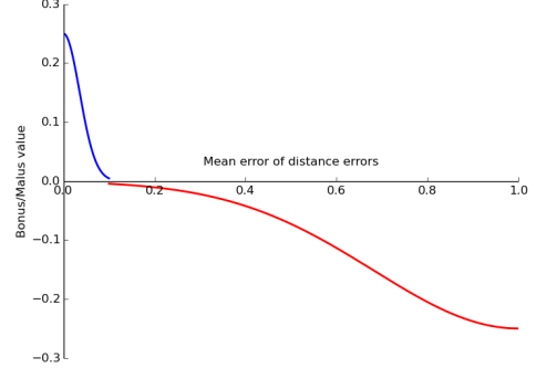
Figure 1: Curves of update values for a static point (blue) and a moving point (red). Here r = 0.25 , \epsilon_{err3D} = 0.10 and max_{err} = 1
