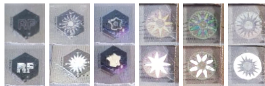
Fig. 7. The counterfeit patterns of the two holograms of the French passport. First row: the scan patterns. Second row: patterns with a glossy sheet.
